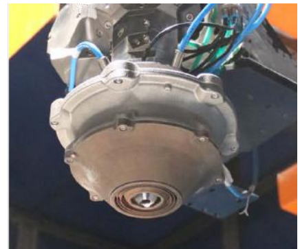
Inert Gas Shielding Nozzle Localized inert atmosphere to process reactive materials (e.g., titanium)
